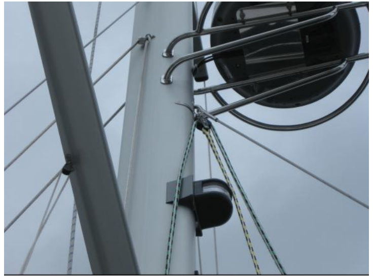
External halyard block installed with becket for fixed length topping lift.
