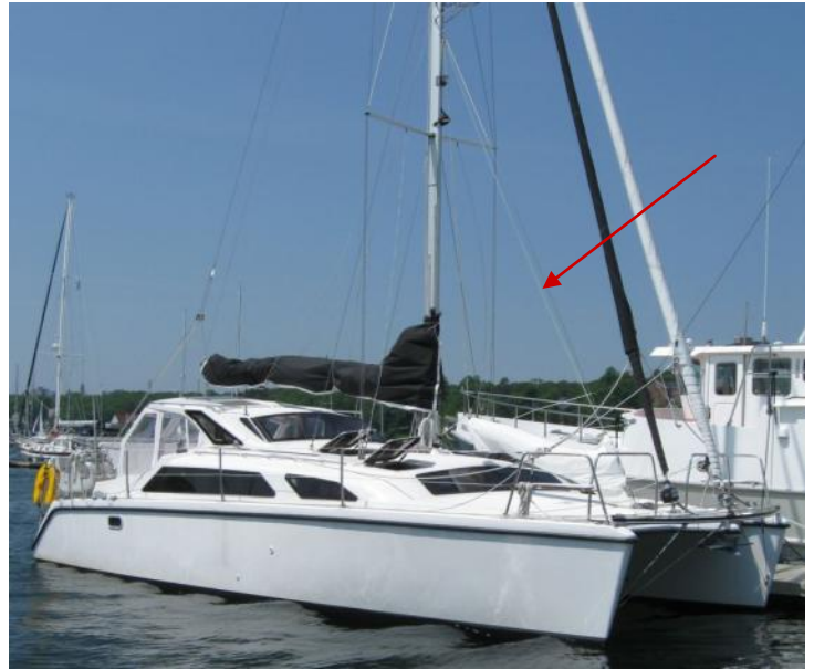
The baby stay modified to attach to the deck about a foot behind the Genoa forestay, creating a foretriangle for the self tacking jib.
