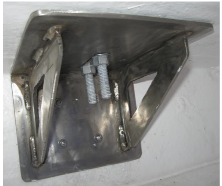
Stainless steel custom bracket in forward center of anchor locker with bottom of deck U bolt shown.
