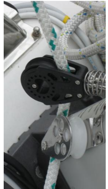
Photo on right: Block on forward face of mast with cheek block below it oriented toward block in photo on left
