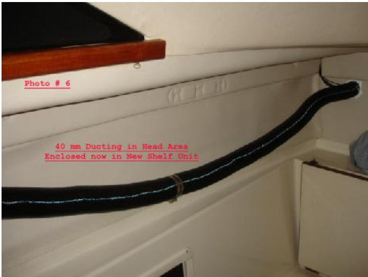
Photo 6. 40 mm ducting in the head. It was later hidden in a new shelf unit.
